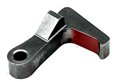
You should remove a small amount of material at a time (a few thousandths) and keep the surface even left to right and top to bottom. After removing some material try it in the gun again.
