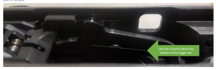
The left side should be adjusted as well but it should barley stay popped out from under the trigger bar. If it comes to rest higher than in the picture you may have to push it down. The left side having too much tension will result in a false reset (an extra audible click when letting the trigger back out for a single action shot).
