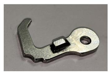
You can also deburr the sides of the disconnector and polish the bottom of the hook that rides on the frame as you pull the trigger. Do not sand or polish on the area that protrudes out the side of the disconnector. Removing material from that area can result in stacking.
