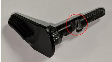
The first area is on the decocker lever in the notch that the sear passes through while pulling the trigger. With the slide off the gun you can pull the trigger and watch the sear contact the edge circled in the pictures. Sometimes the sleeve that hold the decocker spring in place covers part of the cutout. If this it the case for your gun you should file the sleeve back to the edge of the cutout.
